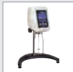
DV1 • Optional Temp Probe • Calculates Viscosity • Torque
