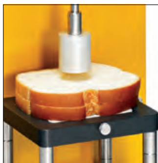
TA-AACC36 F AACC spec probe for measuring bread firmness and performing texture profile analysis (TPA). Fixture Base Table required.
