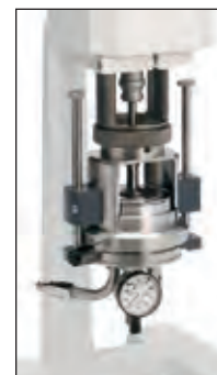
RSS-90Y Spindle for BU measurements on joint compound and similar materials
