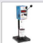
KU-2 Viscometer • KREBS Viscosity • Required for Paint and Coatings
